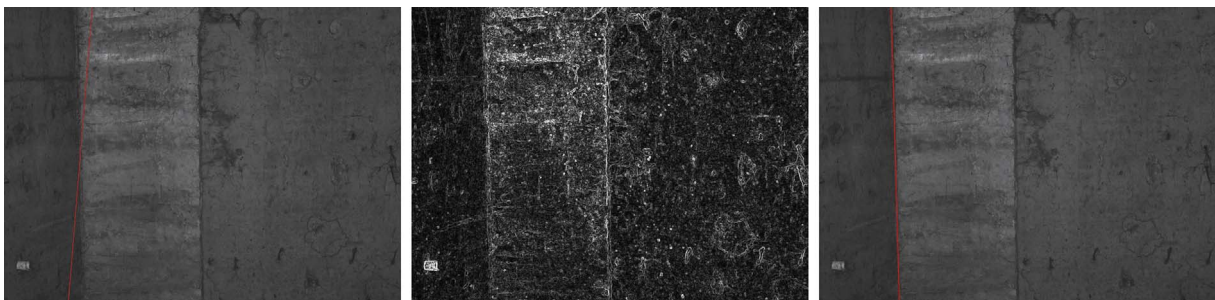
Fig. 6. An example of the obvious structure line in an image: (Left) the initial structure line generated by projection with the rough pose of the image; (Middle) the image gradient map; (Right) the refined structure line optimized by image gradients. The red lines represent the bridge structure lines.
