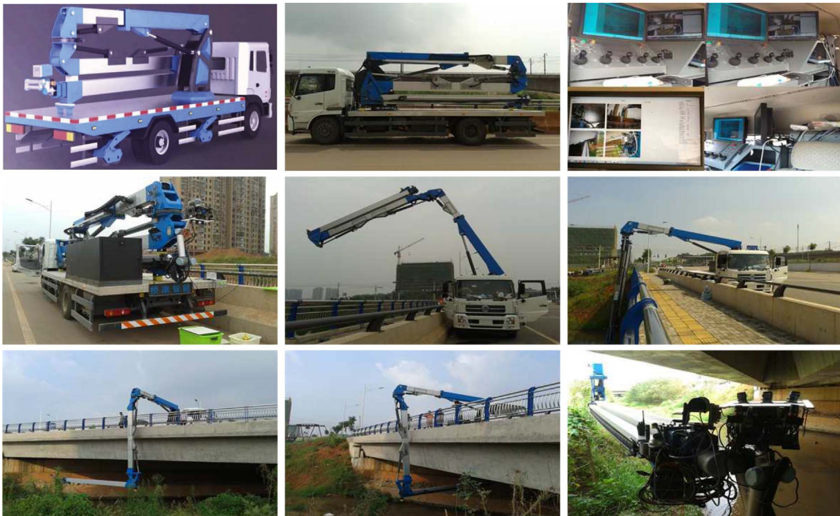
Fig. 10. The design drawing and real photos of the bridge inspection robot system: the design drawing (Left), a real photo in the entire trunk (Middle) and a real photo in the cab control space (Right) in the top row, and six photos captured during working for data acquisition of a test bridge in the middle and bottom rows.
